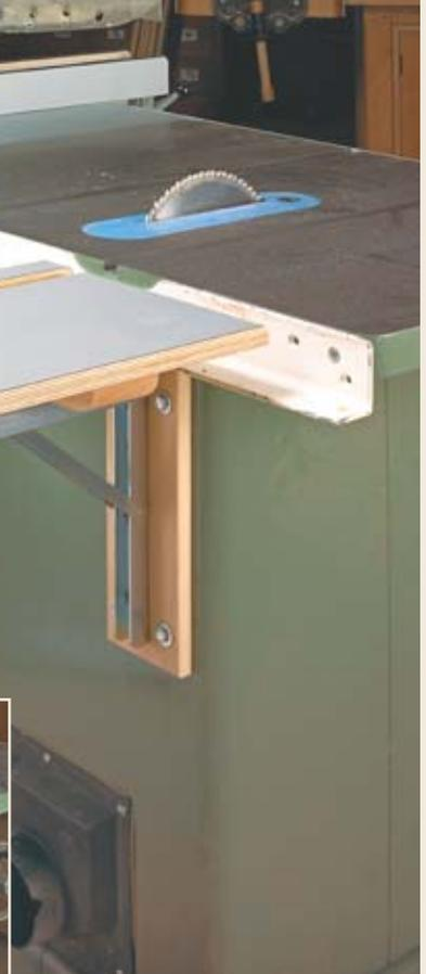
▶ This outfeed extension table swings into action when it's needed and safely tucks out of the way when it's not.
