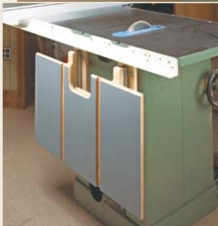
▶ This outfeed extension table swings into action when it's needed and safely tucks out of the way when it's not.
