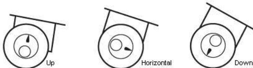
You may wish to use the flexibility of the honing guide and angle jig combination to produce a cutting edge to exactly match the conditions you are working with. In general, you want to sharpen any woodworking chisel or plane blade at the lowest possible angle consistent with the strength of the steel and the intended use of the tool. If you think of the tool as a wedge, you know that a gently tapered wedge penetrates material more easily than a sharply tapered one. More force is spent in
