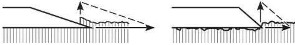
There is a practical limit to reducing the bevel angle. It is determined by the strength of the steel in the tool. You only reduce the angle to the point where the edge will not crumble or bend in use. This angle is usually between 15° and 20° for light paring. Since even tools from the same batch and same manufacturer can vary slightly in hardness, the lowest practical angle will vary from tool to tool.
