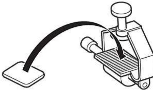
The pad will cover the alignment guide lines on the honing guide so the alignment of narrow chisels should be checked with a small square (as shown in the diagram) using the rear face of the guide as a reference source.
