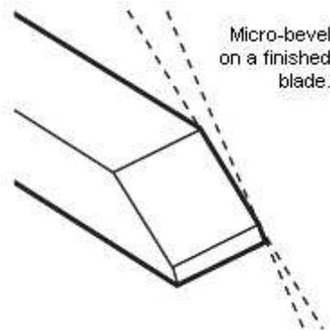
To hone a secondary bevel, turn the setting knob so that the arrow points forward (for a 1° difference) or down (for a 2° difference) and transfer to your finishing stone. A secondary bevel of 1/16" is sufficient. The table below shows the angle of the secondary bevel at specific positions of the setting knob.
