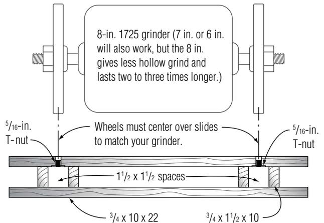
Make of hardwood and run the grain vertically on the sides.
