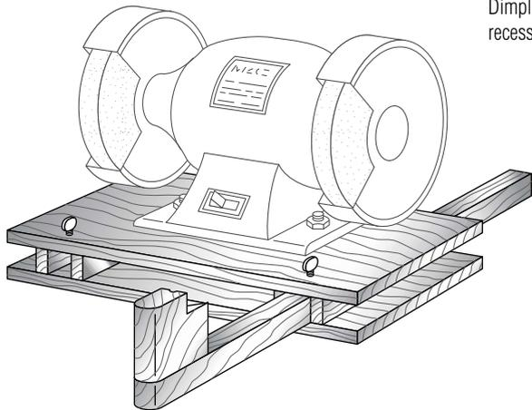
The only metal parts on the jig are two 5/16-in. T-nuts and matching thumbscrews.
